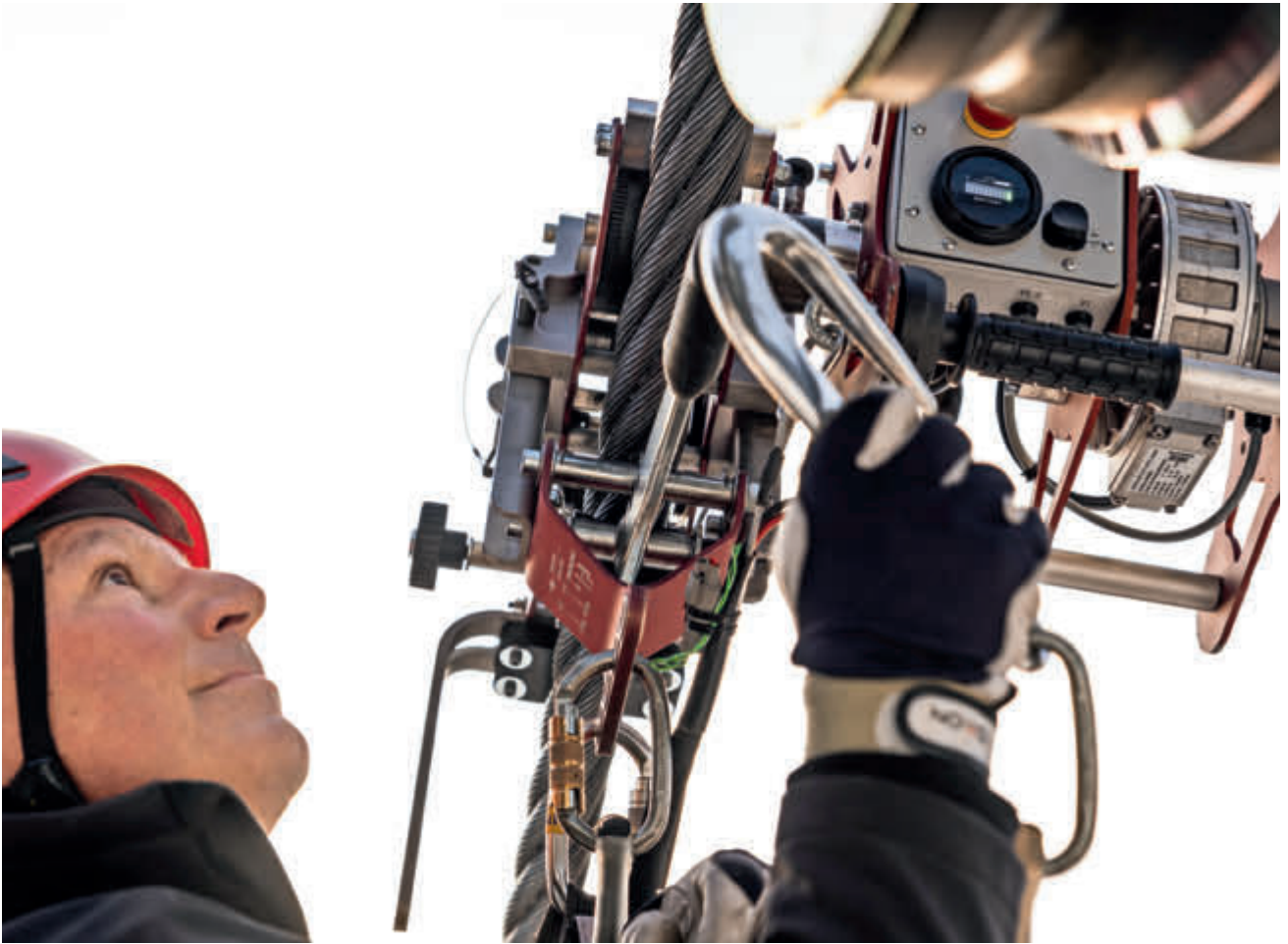
The EDS electric drive is quickly connected to the SS40 AWD cable carriage.
