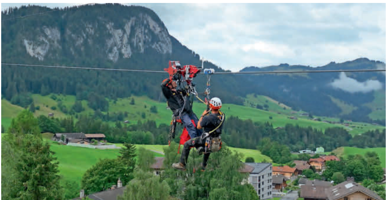
Evacuation training provided by Immoos in Vercorin, Valais, using a combination of SS40 AWD cable carriage, EDS electric drive and the Immoos CS 141 evacuation harness
