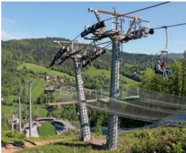
This Leitner double chairlift, which is used for the ski jump in Wisla (PL) in winter and by visitors in summer, will be replaced this year by an inclined elevator, also from Leitner.
