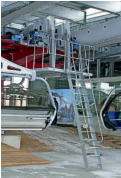
Access and platform for servicing the brakes on the bullwheel of an overhead drive
