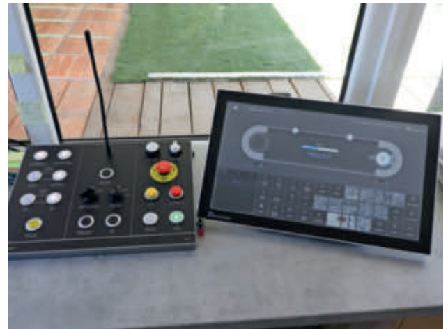
Doppelmayr Connect control system in the bottom station
