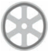
Figure 5: Polygonality in a sheave, e.g. caused by lack of stiffness in the rim
