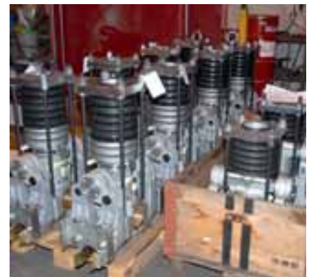
The visit to the Garaventa plant provided an opportunity to inspect the track rope brakes for the 240 t funicular for the Limmern power plant.
