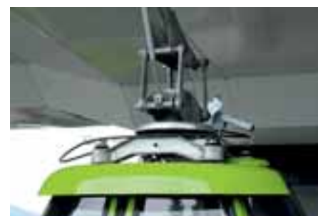
The rotation system on the cabin roof is set to cause the gondola to revolve around its own axis twice during the ride.
