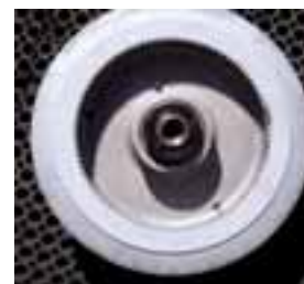
Fig. 3: Timing disc for measuring sheave speed Photos: Hima
